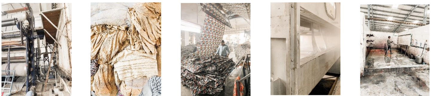
Figure 7: The first image shows a dyeing machine using rolls, it dyes about 2,000 meters of textile per hour. After that the fabric has to go through several finishing processes to bind the dye and soften the textile. The last image shows a finished fabric, 80,000 meters of yellow prints for Mango. Source: (Vonholm, 2019).
